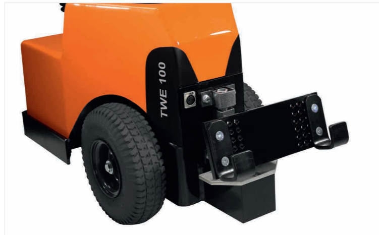
Load connection is easy, with a variety of attachments available.
