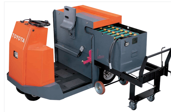
Battery roller bed is standard on CBTY4 model.
