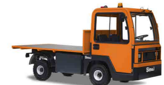
The platform range P15/20/30 ranges from 1500 kg up to 3000 kg. Allows transportation of goods such as maintenance tools or other small cargo.
