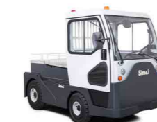
Ideal for heavy-duty airport towing, the TE291 is equipped with sliding doors, inching buttons and a rear platform. It has a towing capacity of 29 tonnes.
