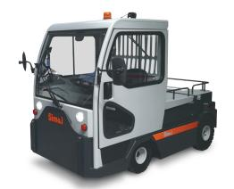
4-wheel tow tractor, man on board, with rear-wheel drive. Ideal for all intense duties - both indoors and outdoors. Loading capacity of wide rear platform 200 kg.
