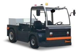
4-wheel tow tractor, man on board, with rear-wheel drive. Heavy-duty high-performance and long-range truck. Loading capacity of wide rear platform 200 kg.
