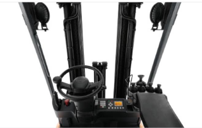
Excellent visibility through the mast with low dashboard including built-in display with essential driver information and functions.
