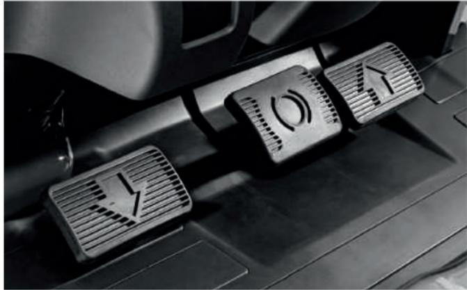
Different pedal layouts to suit driver preference. (Double pedal layout option shown)
