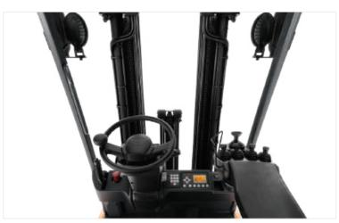
Excellent visibility through the mast with low dashboard including built-in display with essential driver information and functions.
