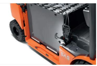
Battery mounted on optional rollerbed for easy extraction.
