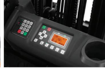
Multifunction display gives key information at a glance, and allows the parameter settings to be adjusted to suit the needs of the application.
