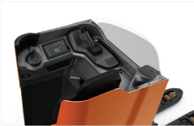
Ergonomic workstation with adjustable and intuitive controls, including a new colour touchscreen display.
