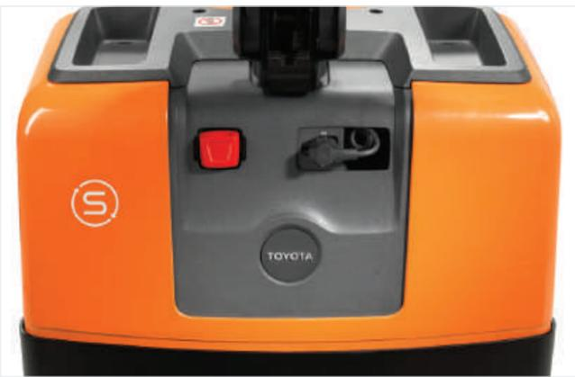
The control panel includes a pull-out power lead for the built-in battery charger.
